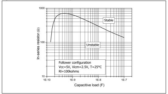
Figure 16. In-series resistor vs. capacitive load
