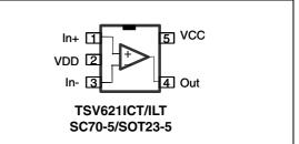
This operational amplifier is unity gain stable for capacitive loads up to 100 pF.
