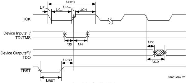
Figure 5. Standard JTAG Timing
