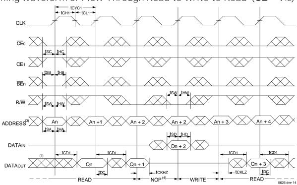
Timing Waveform of Flow-Through Read-to-Write-to-Read (**OE** Controlled)<sup>(2)</sup>
