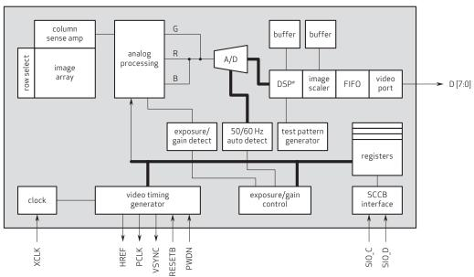
**note 1** DSP\* (lens shading correction, white/black pixel correction, auto white balance, etc.)
