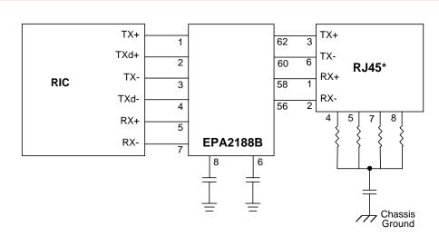
Notes: \* Pin-outs shown are for multiport, DCE configurations: e.g. Hubs, Repeaters
