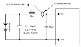
NOTE: Measure input reflected ripple current with a simulated source inductance (L<sub>TEST</sub>) of 12µH. Capacitor C<sub>S</sub> offsets possible battery impedance. Measure current as shown above
