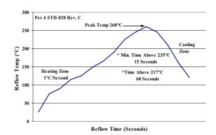
Figure 19. Recommended linear reflow profile using Sn/Ag/Cu solder.
