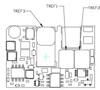
Figure 13.  $T_{ref}$  Temperature Measurement Locations.
