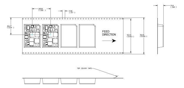
The Sixteenth-brick SMT versions are supplied in tape & reel as standard. Details of tape dimensions are shown above. Modules are shipped in quantities of 140 modules per reel.
