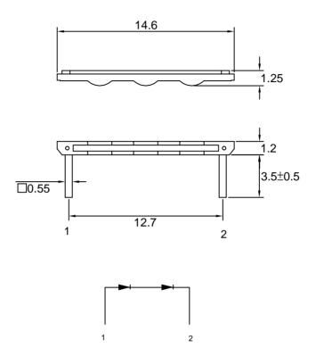
Note : 1.All dimension are in millimeter tolerance is  $\pm 0.25$ mm unless otherwise noted.
