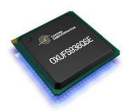
The OXUFS936QSE is a universal interface (eSATA, FireWire800, FireWire400, USB2.0) to quad SATA storage controller. Delivering industry leading performance across all interfaces, the OXUFS936QSE supports a range of 4-disk and 3-disk RAID configurations and provides a platform for OEMs to develop a range of external storage systems.
