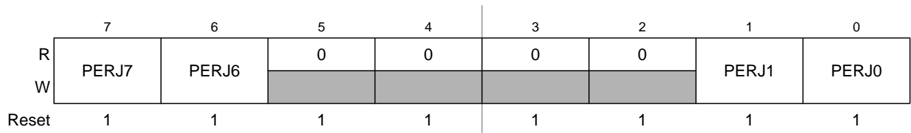
Figure 2-60. Port J Pull Device Enable Register (PERJ)
