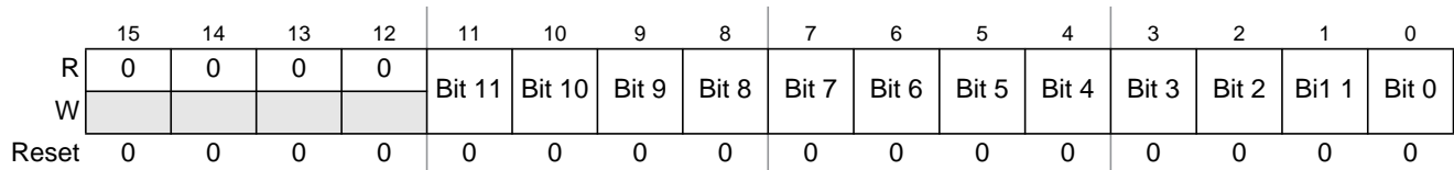
Figure 10-15. Right justified ATD conversion result register (ATDDR n )
