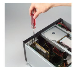
User-friendly mechanical design for installing an add-on card
