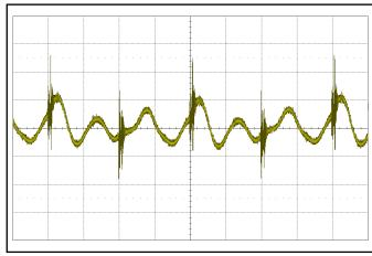
Figure 14: Output voltage ripple at nominal input voltage and rated load current (50 mV/div; 2 µs/div). Load capacitance: 1 µF ceramic capacitor and 15 µF tantalum capacitor. Bandwidth: 20 MHz. See Figure 11.
