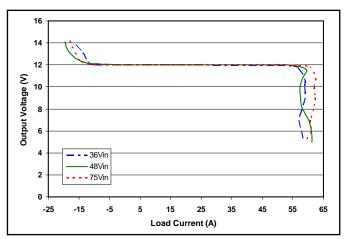
Figure 17: Output voltage vs. load current showing typical current limit curves and OVP shutdown point.
