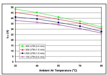
Figure 3: Maximum output power derating curves vs. ambient air temperature for airflow rates of 100 LFM through 400 LFM with air flowing across the converter from pin 4 to pin 1 (nominal input voltage).
