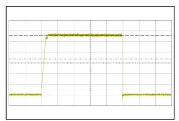
Figure 16: Load current (10 A/div; 10 ms/div) as a function of time when the converter attempts to turn on into a 1 m $\Omega$  short circuit.
