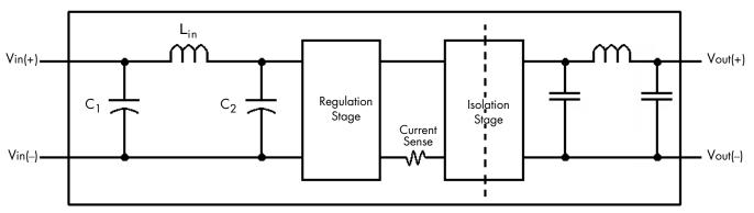
Figure F: Internal Input and Output Filter Diagram (component values listed on specifications page).
