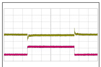
Figure 10: Output voltage response to step-change in load current (50%-75%-50% of Iout(max):  $dI/dt = 5 A/\mu s$ ; 1 ms/div). Load cap: 470  $\mu F$ , 15 m $\Omega$  ESR electrolitic capacitor. Top trace: Vout (500 mV/div). Bottom trace: Iout (10 A/div).
