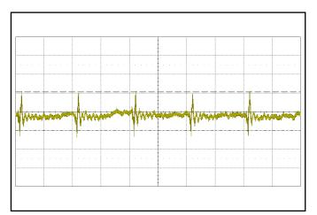
**Figure 13:** Input reflected ripple current,  $i_s$ , through a 4.7  $\mu$ H source inductor, using a 220  $\mu F$  input capacitor, at nominal input voltage and rated load current (10 mA/div; 2 µs/div). See Figure 11.
