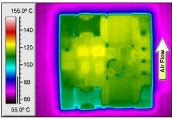
Figure 4: Thermal plot of converter at 36 A load current (432 W) with 55°C air flowing at the rate of 200 LFM. Air is flowing across the converter sideways from pin 4 to pin 1 (nominal input voltage).
