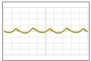
Figure 12: Input Terminal Ripple Current, ic, at full rated output current and nominal input voltage with 4.7 µH source impedance and 220 μF electrolytic capacitor (1 A/div; 2 μs/div). See Figure 11.
