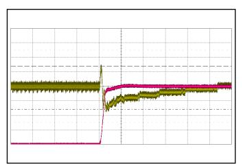
Figure 15: Output voltage response to step-change in input voltage (35 V to 75 V in 300  $\mu$ s; 1 ms/div). Load cap: 470  $\mu$ F, 15 m $\Omega$  ESR electrolitic capacitor. Top trace: Vout (500 mV/div). Bottom trace: Vin (10 V/div), at zero load current.
