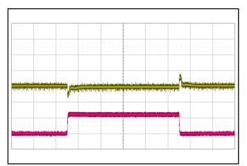
Figure 9: Output voltage response to step-change in load current (50%-75%-50% of Iout(max); dI/dt = 0.1 A/ $\mu$ s; 1 ms/div). Load cap: 1  $\mu$ F ceramic and 470  $\mu$ F, 15  $m\Omega$ ESR electrolitic capacitors. Top trace: Vout (500 mV/div). Bottom trace: Iout (10 A/div).
