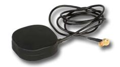
The RF-3070-AT242 is a portable, active L1/L2 GPS antenna with an integrated pendant coaxial cable and magnetic mount. The 3-foot long RG-174 coaxial cable terminates in a right angle SMB connector for direct connection to the AN/PRC-117G(V)1(C) and RF-7800M-MP Falcon III® manpack transceivers. The magnetic mount has a retaining force of approximately 18 lbs.
