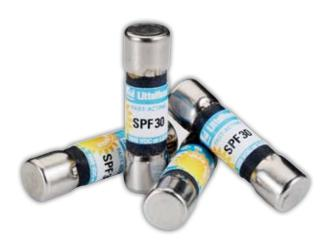
The SPF Solar Protection Fuse series has been specifically designed for photovoltaic (PV) systems. This family of midget fuses (10x38mm) can safely protect PV modules and their conductors from reverse overcurrent conditions despite the associated challenges of DC power.
