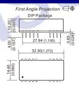
RECOMMENDED FOOTPRINT Top view,grid:2.54mm(0.1inch) diameter:1.00mm(0.039inch)
