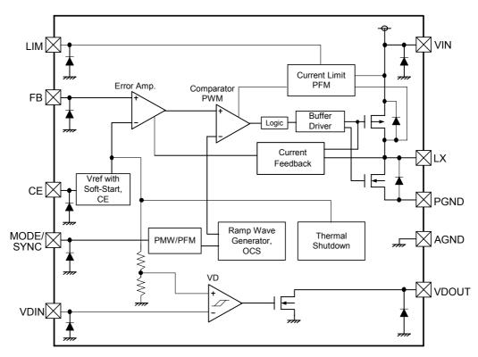
1A Driver Transistor Built-In Step-Down DC/DC Converters
