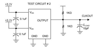
For parameter  $t_{\text{8}}$  (output skew rate) on -1H devices
