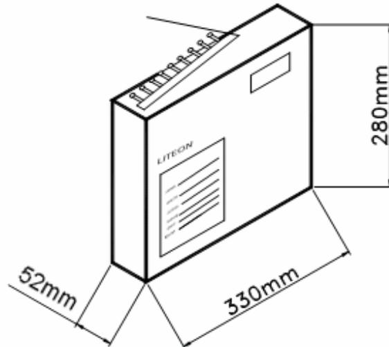
Tolerance:  $\pm 5\text{mm}$ **10 Inner cartons per outer carton****total 20000 pcs per outer carton****In every shipping lot, only the last pack will be non-full packing**
