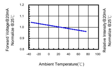
Fig.4 Relative Intensity vs. Temperature
