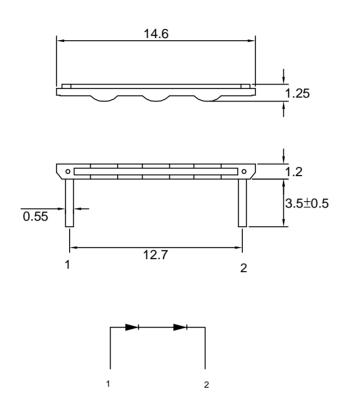
Note : 1.All dimension are in millimeter tolerance is  $\pm 0.25$ mm unless otherwise noted.
