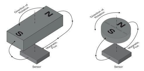
The sensor element free layers will align with the external field. As the applied field changes direction, the angle between the free layer and the pinned layer changes, changing the resistance of TMR elements, which changes the device output voltages.
