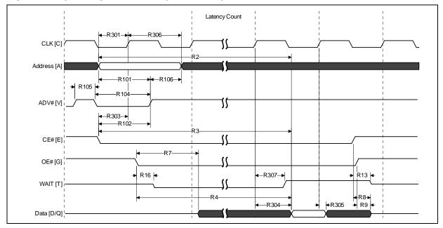
Figure 22: Sync Single-Word Array/Non-Array Read, 108 MHz
