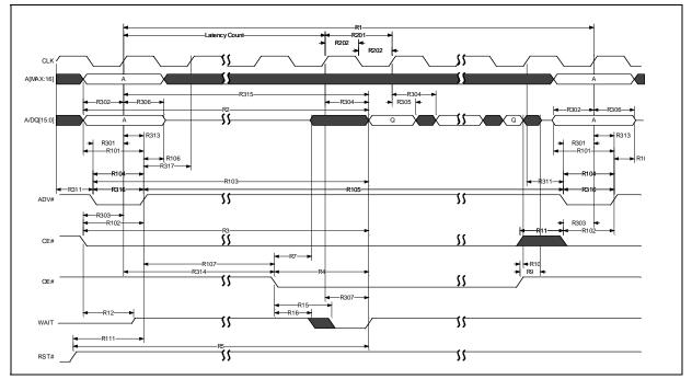
Figure 29: Synchronous Burst with Burst-Interrupt (AD-Mux)
