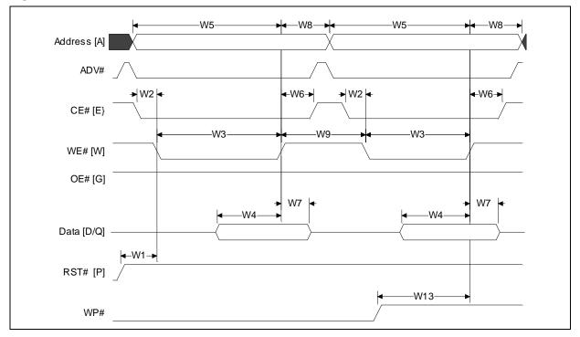
Figure 30: Write to Write (Non-Mux)
