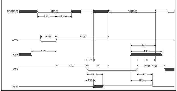
Figure 62: AADM Asynchronous Read Cycle (Latching A[15:0] only)
