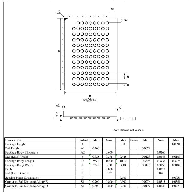
Figure 6: Mechanical Specifications: x16C (107-ball) package (8x10x1.0 mm)
