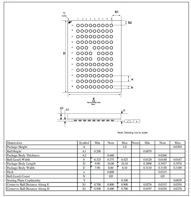
Figure 1: Mechanical Specifications: x16D (105-ball) package (8x10x1.0 mm)
