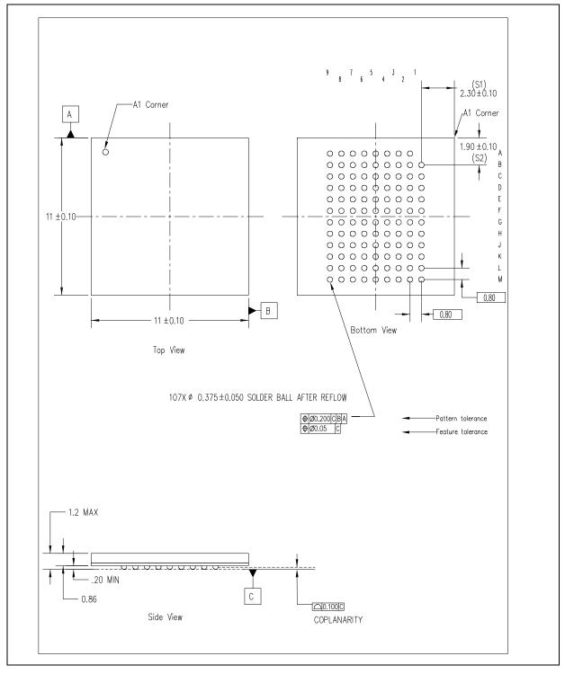
Figure 9: Mechanical Specifications: x16C (107-ball) package (11x11x1.2 mm)
