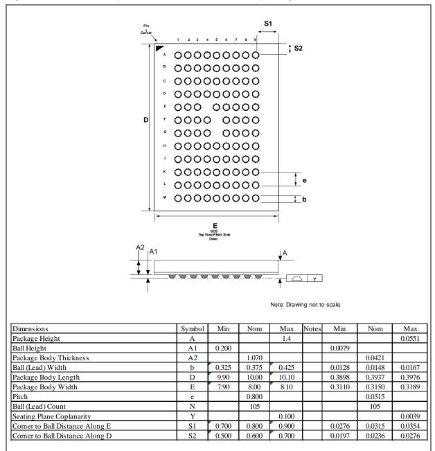
Figure 2: Mechanical Specifications: x16D (105-ball) package (8x10x1.4 mm)
