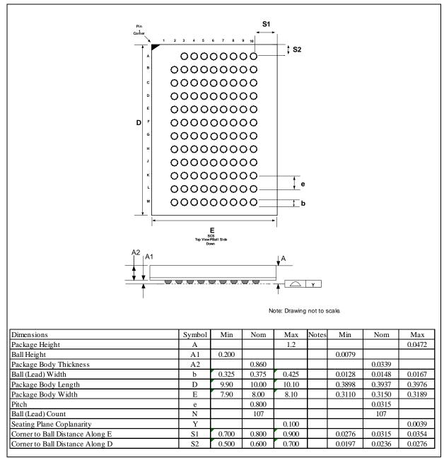
Figure 7: Mechanical Specifications: x16C (107-ball) package (8x10x1.2 mm)
