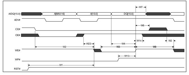
Figure 64: AADM Asynchronous Write Cycle (Latching A[15:0] only)
