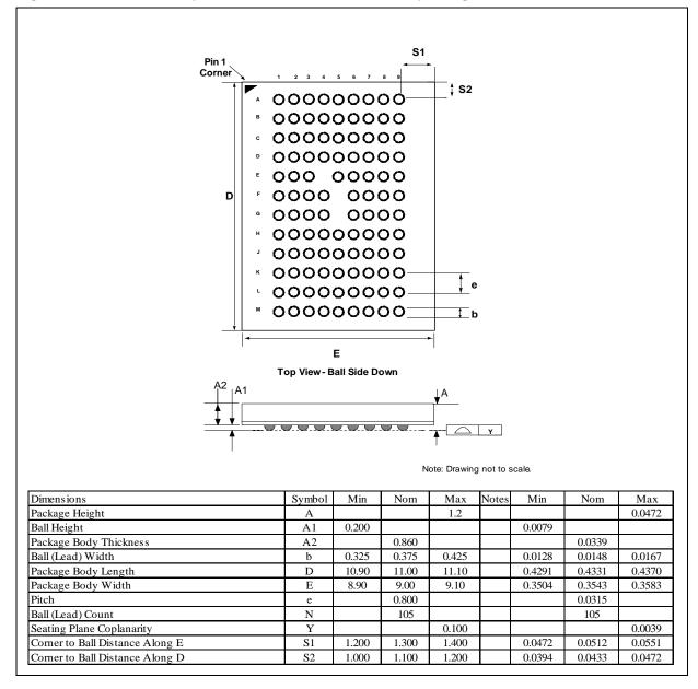
Figure 3: Mechanical Specifications: x16D (105-ball) package (9x11x1.2 mm)
