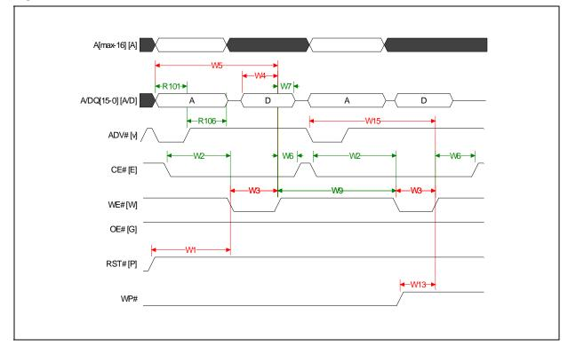
Figure 35: Write to Write (AD-Mux)
