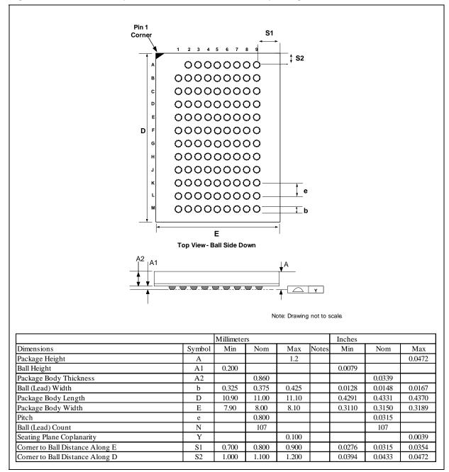
Figure 8: Mechanical Specifications: x16C (107-ball) package (8x11x1.2 mm)
