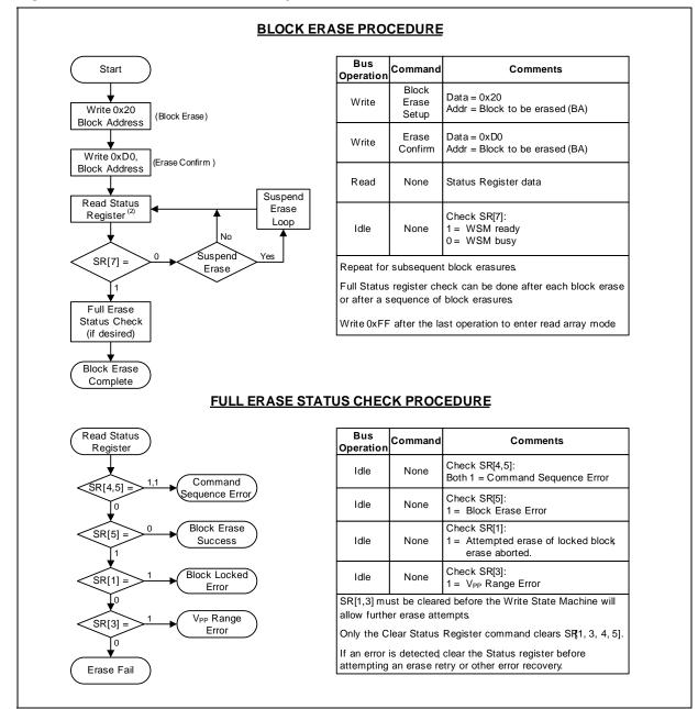
Figure 56: Block Erase for Main Array Flowchart
