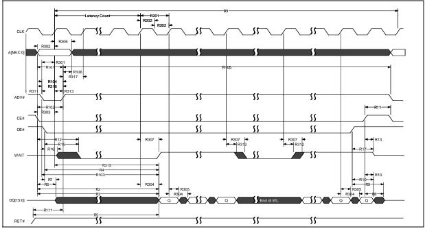
Figure 24: Synchronous Continuous Mis-aligned Burst (Non-Mux)
