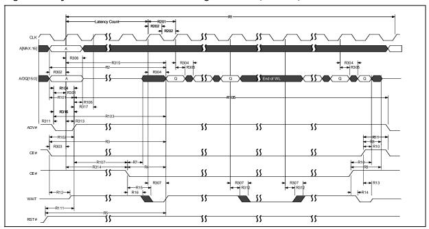
Figure 28: Synchronous Continuous Mis-Aligned Burst (AD-Mux)
