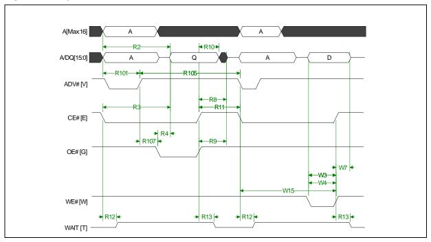
Figure 36: Async Read to Write (AD-Mux)
