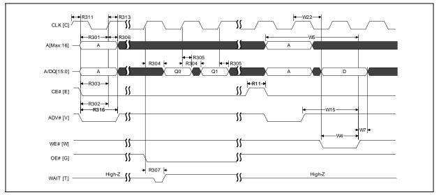
Figure 38: Sync Read to Write (AD-Mux)
