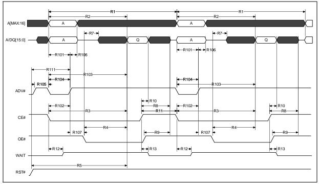
Figure 26: Async Single-Word Read (AD-Mux)
