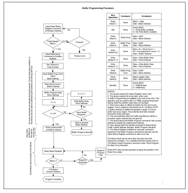
Figure 54: Buffered Program Flowchart
