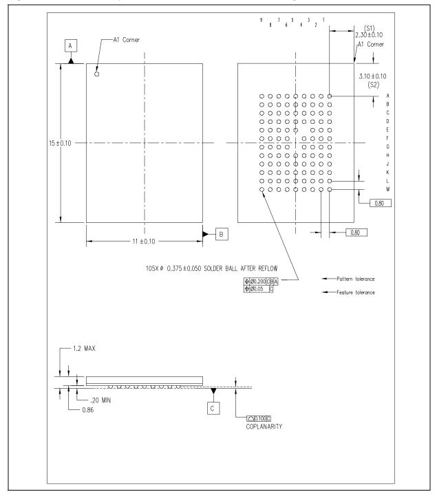
Figure 4: Mechanical Specifications: x16D (105 balls) Package (11x15x1.2 mm)
