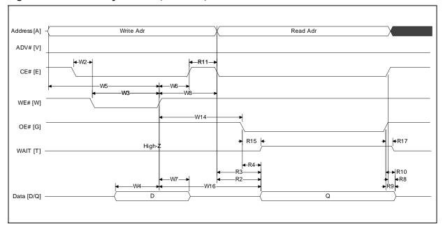
Figure 32: Write to Async Read (Non-Mux)
