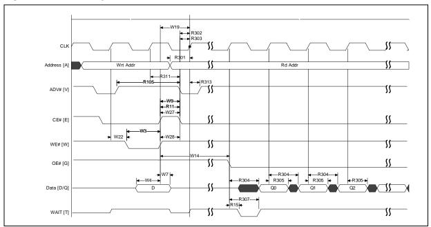
Figure 34: Write to Sync Read (Non-Mux)
