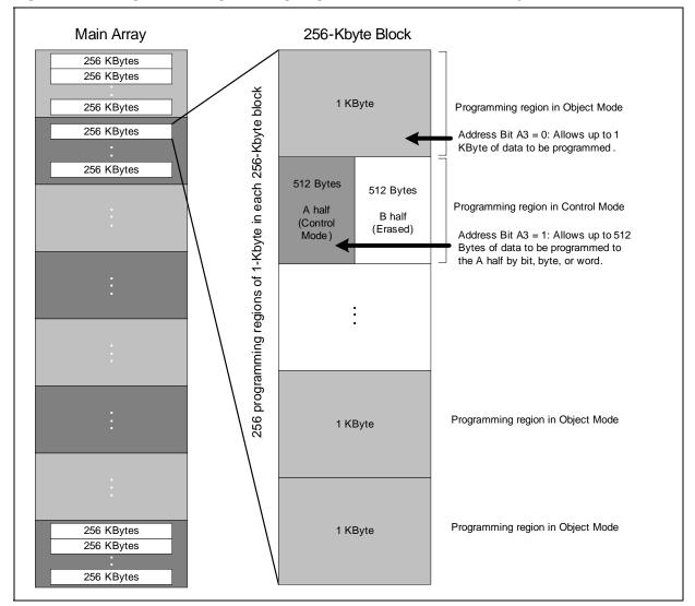
Figure 47: Configurable Programming Regions: Control Mode and Object Mode
