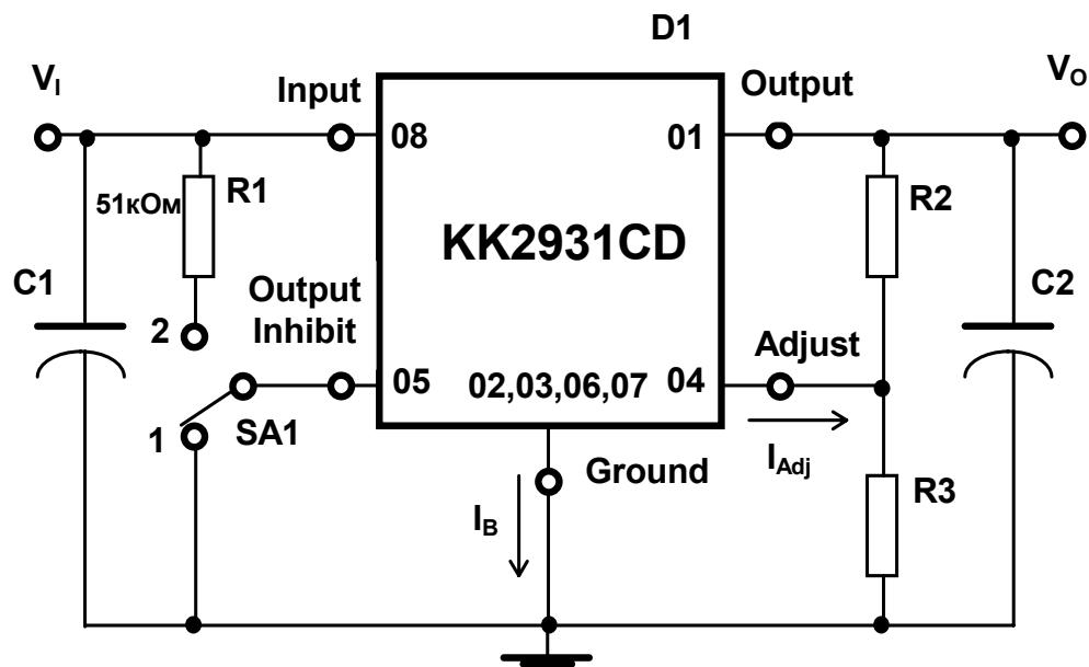
C1, C2 - input and output capacitance,
