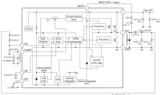
C1,C8,C5,C9 = Ceramic capacitor L1=CDRH105RNP-100NC(sumida)
