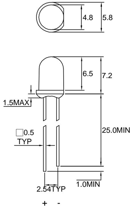
Note : 1.All dimension are in millimeter tolerance is  $\pm 0.25\text{mm}$  unless otherwise noted.
