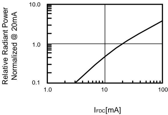
Fig.4 Relative Radiant Power vs. Forward Peak Current
