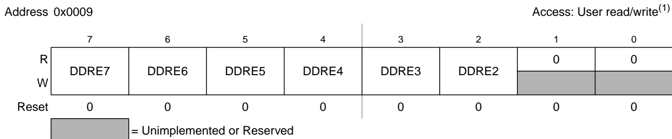
Figure 2-7. Port E Data Direction Register (DDRE)
