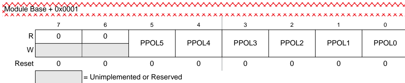
Figure 10-4. PWM Polarity Register (PWMPOL)
