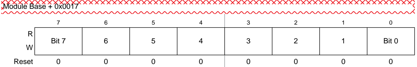
Figure 10-26. PWM Channel Period Registers (PWMPER5)
