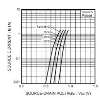
Fig.5 Source Current vs. Source-Drain Voltage
