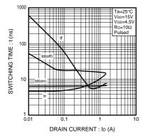
Fig.1 Switching Characteristics
