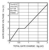
Fig.2 Dynamic Input Characteristics
