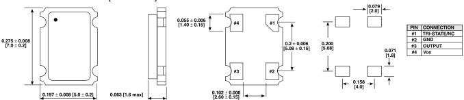
\*\*\*note: A 0.01  $\mu$ F bypass capacitor should be placed between VDD(Pin4) and GND(Pin2) to minimize power supply line noise
