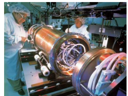
Telecommunications Undersea Cable Repeater
