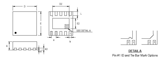
Note: The configuration of the Pin #1 identifier is optional, but must be located within the zone indicated.
