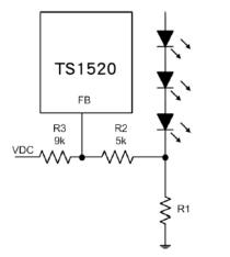
Figure 1. Dimming Control Using a DC Voltage
