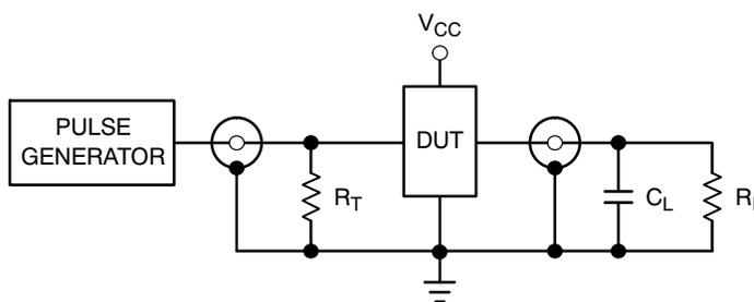
$R_T = Z_{OUT}$  of pulse generator (typically 50  $\Omega$ )
