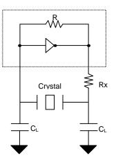
$C_L = 2^*(C_P - C_S), \\ Where C_P = Load capacitance of crystal \\ C_S = Stray capacitance due to C_{IN,} PCB, Trace etc.$
