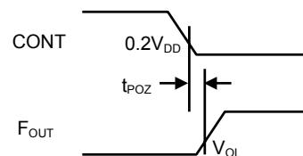
(3)Output Enable Time ( $C_L=5\text{pF}$ )
