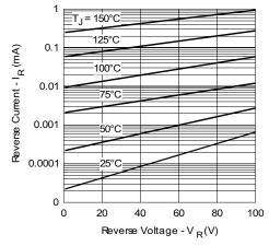
Fig. 2 - Typical Peak Reverse Current vs. Reverse Voltage
