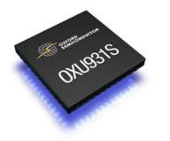
The OXU931S is a single chip solution for bridging between USB2.0 and hard disks. Optimized for performance and low cost of ownership, the OXU931S is ideal for creating external storage devices which connect to a PC or Mac via the USB2.0 port.
