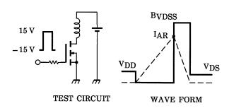
$$\begin{aligned} &R_G = 25~\Omega \\ &V_{DD} = 25~V,~L = 11.6~mH \end{aligned} \qquad E_{AS} = \frac{1}{2} \cdot L \cdot I^2 \cdot \left( \frac{B_{VDSS}}{B_{VDSS} - V_{DD}} \right) \end{aligned}$$
