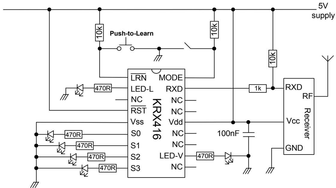
Figure 2: KRX416 Function-Code display - example circuit
