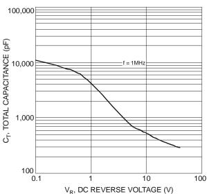
Fig. 3 Total Capacitance vs. Reverse Voltage
