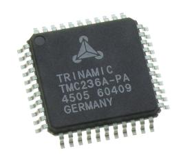
INFO The TMC236 is a smart power microstepping driver for bipolar stepper motors. It provides an SPI™ interface as well as the classical analog/digital control. A full set of protection and diagnostic features makes this device very rugged. The integrated low-RDS-ON TrenchFET<sup>®</sup> power MOSFETs give an extremely high efficiency and allow driving of a high motor current of up to 1.5A per phase without cooling measures even at high environment temperatures.
