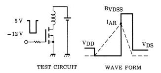
$$\begin{array}{l} T_{ch} = 25^{\circ}C \; (Initial) \\ Peak \; I_{AR} = -6 \; A, \; R_G = 25 \; \Omega \quad E_{AS} = \frac{1}{2} \cdot L \; \cdot I^2 \cdot \; (\frac{BVDSS}{BVDSS - V_{DD}}) \\ V_{DD} = -16 \; V, \; L = 1.0 \; mH \end{array}$$
