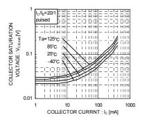
Fig.7 Collector-Emitter Saturation Voltage vs Collector Current  $({\rm I\hspace{-.1em}I\hspace{-.1em}I})$
