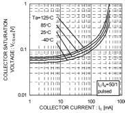
Fig.8 Collector-Emitter Saturation
