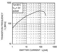
Fig.9 Transion frequency vs Emitter Collector
