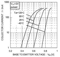
Fig.2 Grounded Emitter Propagation Characteristics
