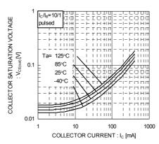
Fig.6 Collector-Emitter Saturation
