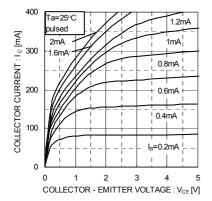
Fig.1 Typical Output Characteristics
