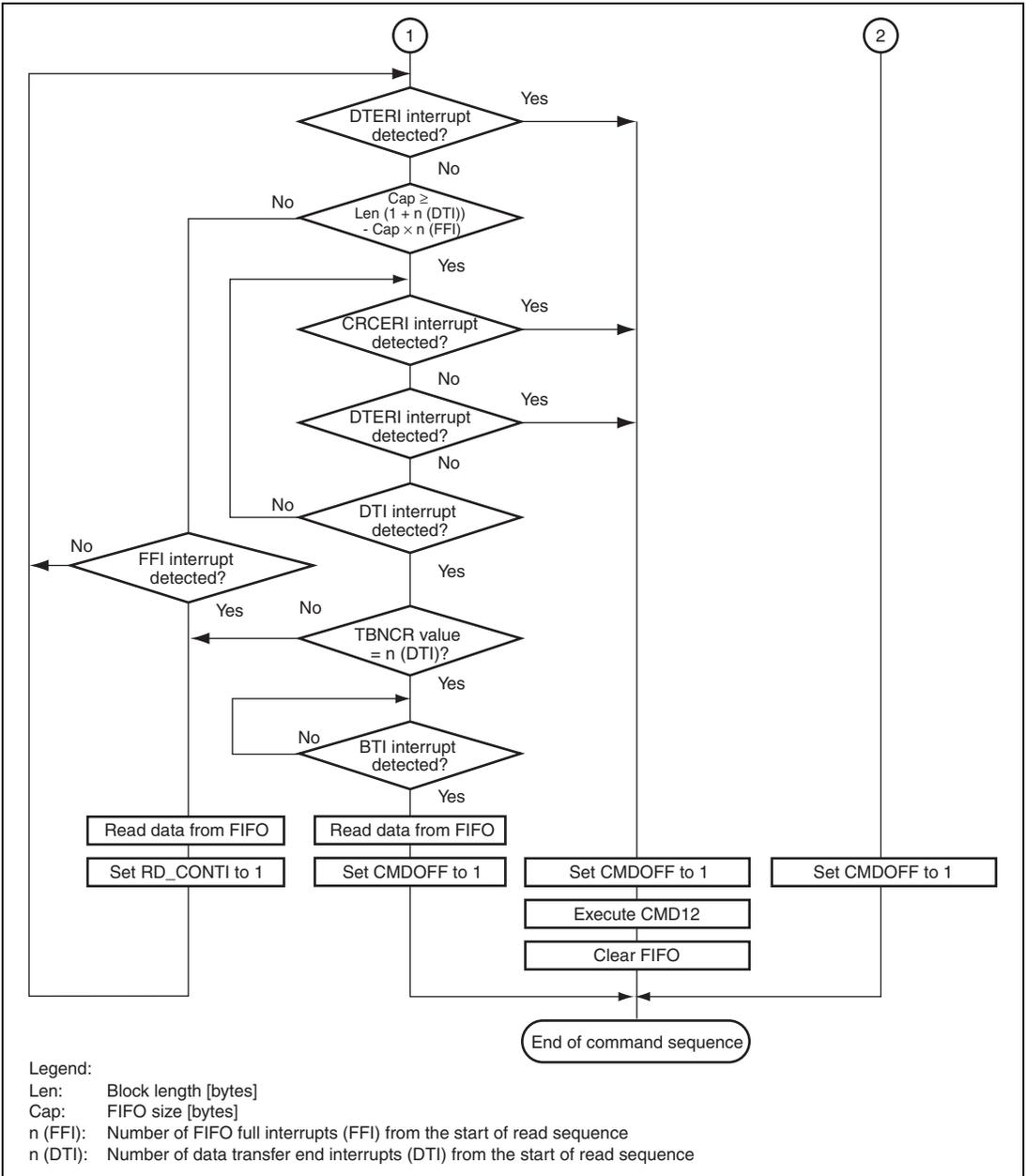
**Figure 24.13 Example of Operational Flow for Commands with Read Data (4)
