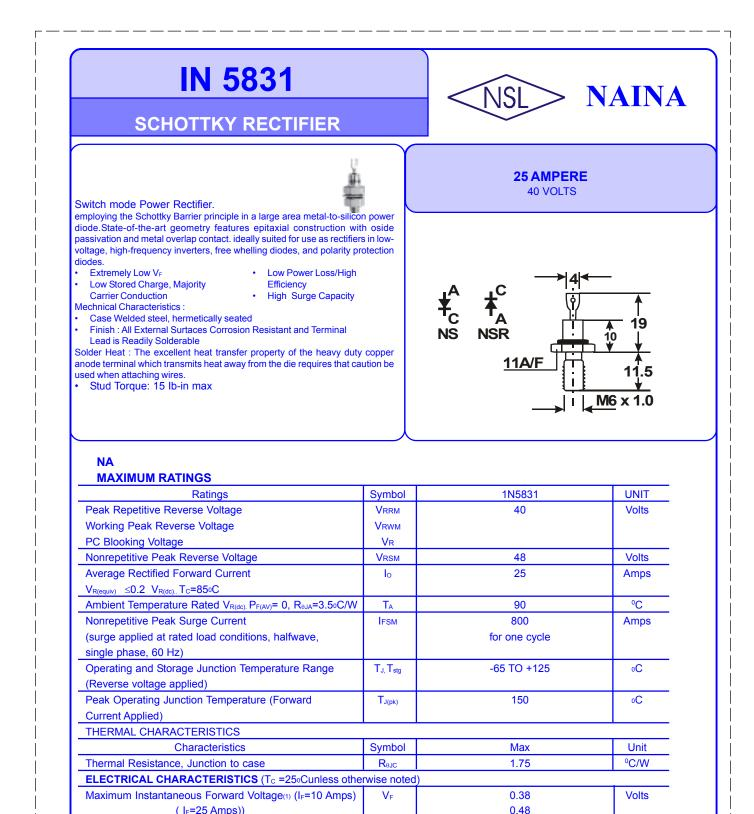
(I⊧=25 Amps)) (I⊧=78.5 Amps) Maximum Instantaneous Reverse Current @ Rated dc Voltage⑴ (1) (Tc=100°C
