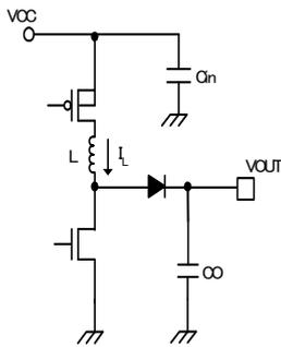
The input capacitor selected should have low ESR with enough capacity to be compatible large ripple current, in order to prevent large transient voltage. The ripple current IRMS can be derived from formula (5).
