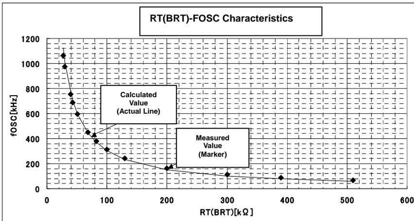
$$f_{osc} = \frac{3.04 \times 10^4}{RT(BRT)[k\Omega]} [kHz]$$
