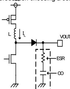
The output ripple voltage is determined by formula (4).
