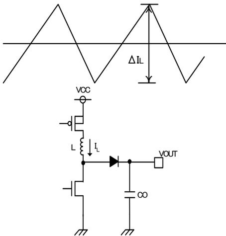
The value of the coil greatly affects the input ripple current. As presented in formula (1), the larger the coil and the higher the switching frequency, the lower the ripple current.
