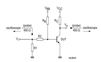
$V_i$  = 0.5 V to 4.2 V; T = 500  $\mu s;$   $t_p$  = 10  $\mu s;$   $t_r$  =  $t_f \leq$  1 ns.
