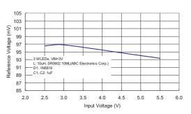
Input Voltage VS Reference Voltage
