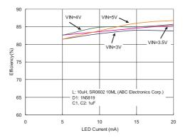
3 WLEDs Efficiency vs. LED Current
