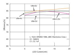
5 WLEDs Efficiency vs. LED Current
