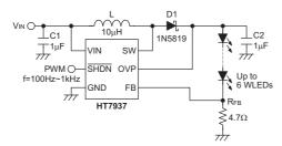
Figure 1. Dimming Control with PWM Signal
