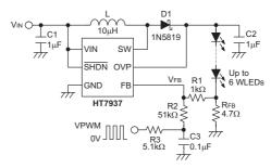
Figure 3. Dimming Control Using a Filter PWM Signal
