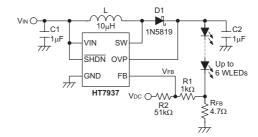
Figure 2. Dimming Control Using a DC Voltage
