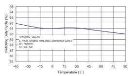
Temperature VS Switching Duty Cycle
