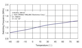
Temperature VS Switching Frequency
