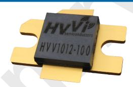
The device resides in a two-lead metal flanged package with liquid crystal polymer lid. The HV400 package style is qualified for gross leak test – MIL-STD-883, Method 1014.
