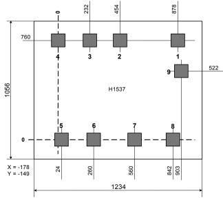
Pad opening 90µm x 90 µm typical.
