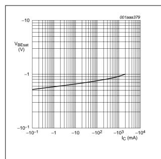
$I_C/I_B = 20$ .  $T_{amb} = 25 \,^{\circ}C$ .
