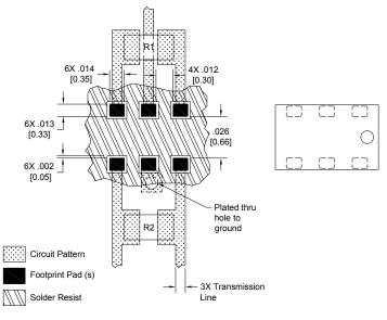
Dimensions are in Inches [Millimeters] Mounting Footprint
