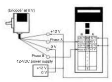
Note: Apply the following connections if the E6C3's 3 power supplies are 5 or 24 V.
