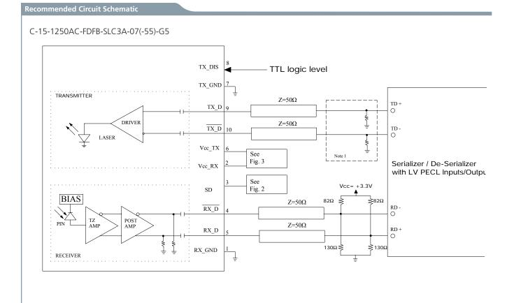
The split-loaded terminations for ECL signals need to be located at the input of devices receiving those ECL signals.
